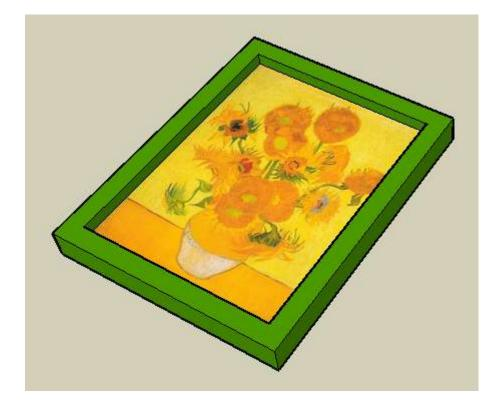
11. Here's a very important step when you're making a model you'll be using later in another model. We need to determine how this painting will align when it's imported into the museum. So choose **Window / Model Info**, and open the **File** page. Next to **Glue to**, choose **Any**. This means when it's imported, the painting will align to any face, whether the face is vertical or horizontal or sloped.
